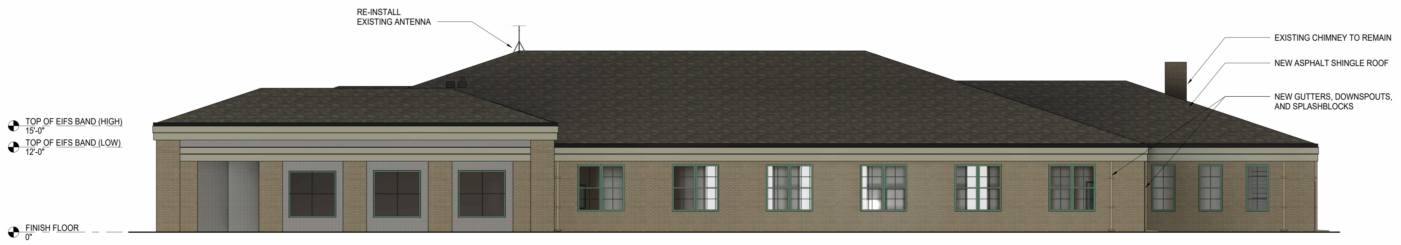
2 EAST ELEVATION - NEW WORK A201 1/8" = 1'-0"
